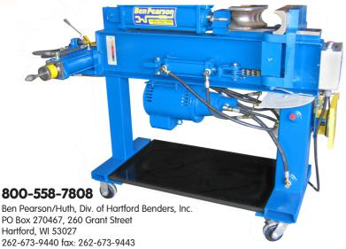
The BP-08 is our new low-cost alternative for shops just starting up, adding exhaust service to their existing business, adding a second bender or replacing an old bender but still using the existing tooling.
