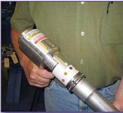
The Huth Model 1685 expander is a popular item for shops that install exhaust but don't have a bender.
