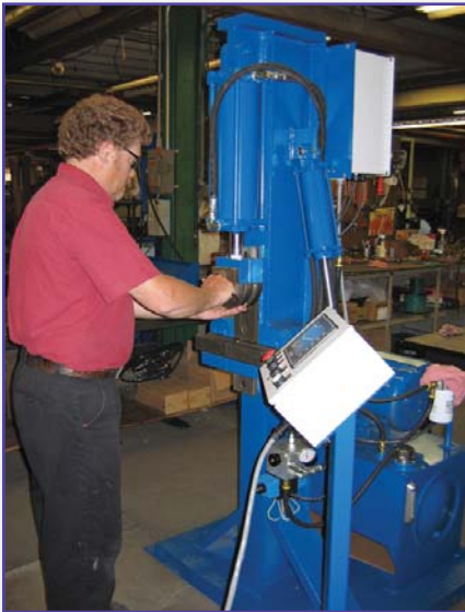
Mark Purman tests Huth's new Model 3002 vertical bender.
