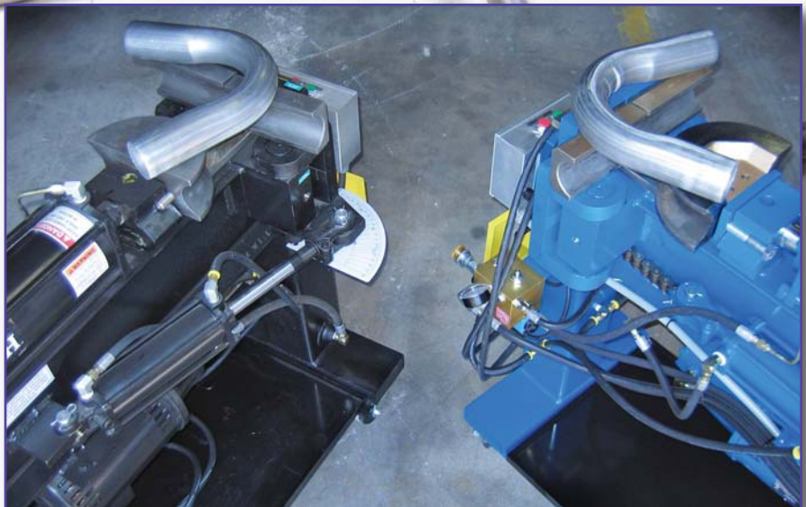
The Huth HB-10 and the Ben Pearson HB-09 both use I-beam frame construction but differ in that the HB-10 uses traditional Huth dies and the HB-09 uses Ben Pearson dies. In addition, the Huth unit uses a hydraulic ram and the Ben Pearson uses a chain drive.
