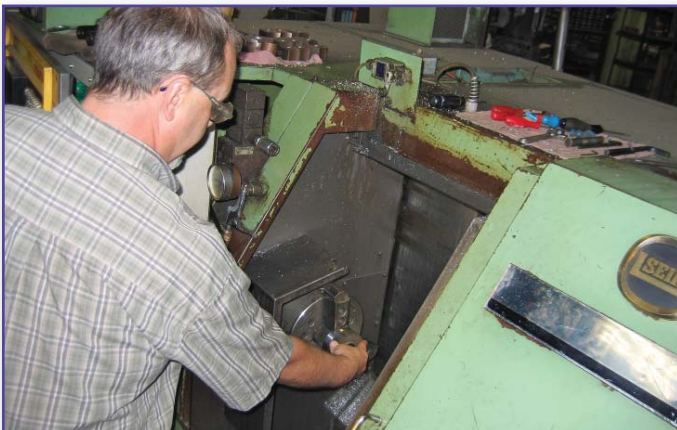
Pete Held uses the company's CNC machine to make bender tooling.
