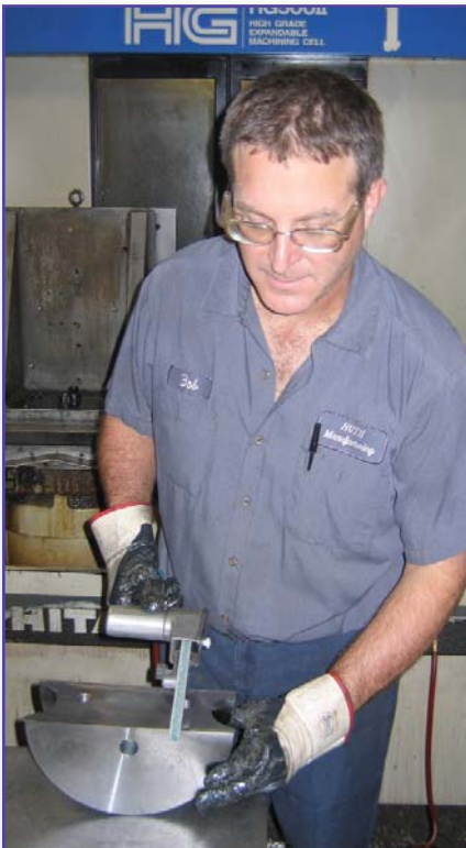
Bob Lechner checks the tolerances on a half-shoe die.
