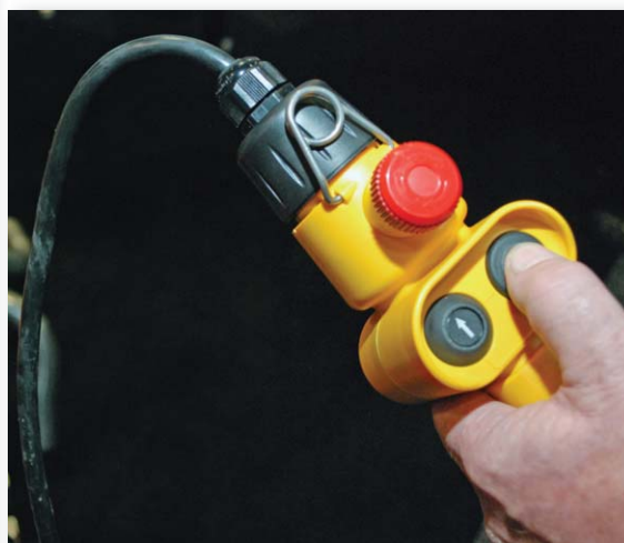
The HB-20 bender and tooling package incorporates an electronic controller tethered to the machine that allows the operator to be as far as 6 feet away from the unit.
