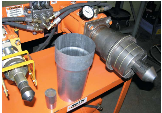
Swaging equipment is designed to expand from 1- to 10-inch tubing.
