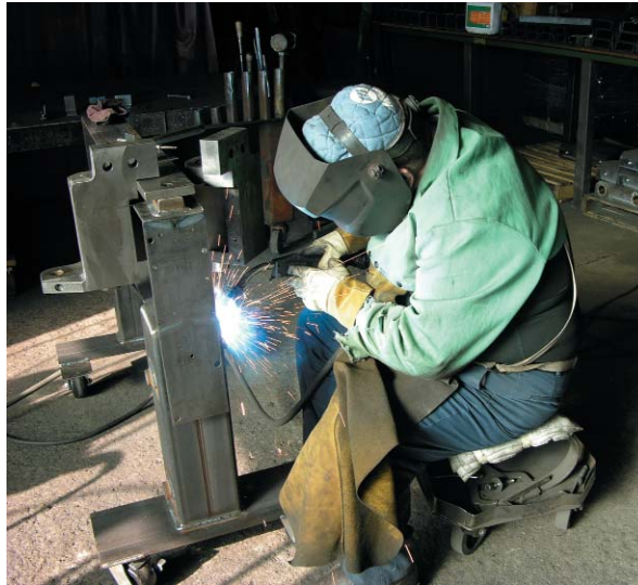
Mark Jeffords welds a sequence-valve mounting bracket onto a bender frame.
