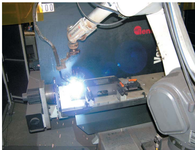
A swager box is welded robotically at the plant.
