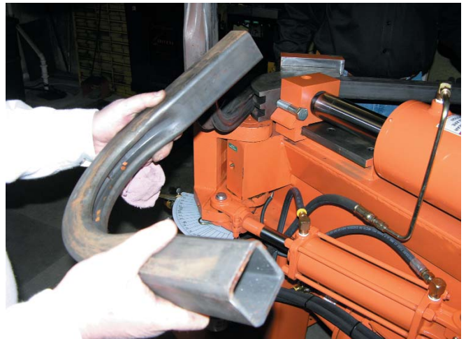
The new 2600 HD model is designed to bend heavy-wall round, square and even some rectangular tubing. Shown is a 2-inch square tube with a \frac{3}{16} -inch wall.
