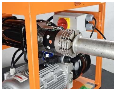
Figure 17. Male V-Band formed
