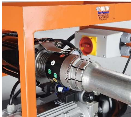
Figure 6. Tubing placement over arbor and segment set
