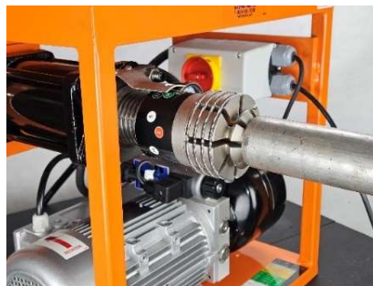
Figure 16. Tube over segment set
