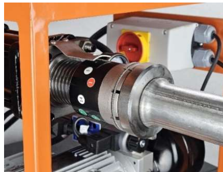
Figure 11. Tubing meets the inside of the flange ring, flange formed
