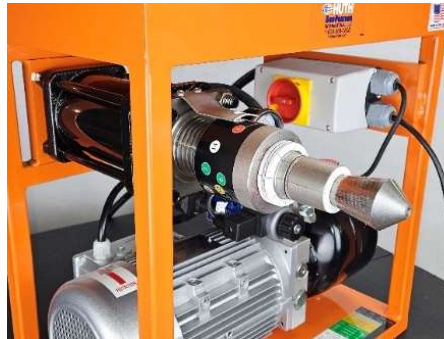
Figure 3. Segment set on the arbor
