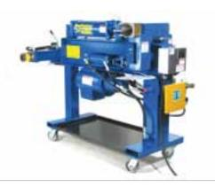
The BP-08 and BPC-09 are manually operated benders using the knee control for bending and I-Beam construction with the maintenance free guide plate. The BPC-09 combination is a low cost alternative for shops just starting out, adding exhaust service or adding additional benders to their operation.
